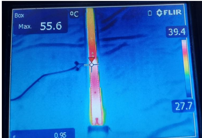
Temperature measurement point on TMP LED
