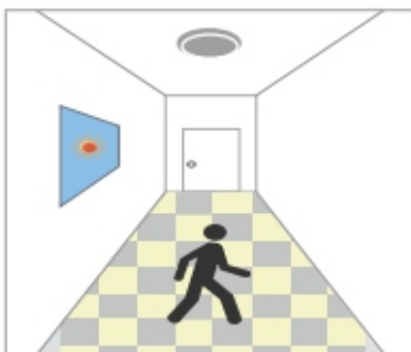
With sufficient daylight, even when motion detected, light remains OFF.
